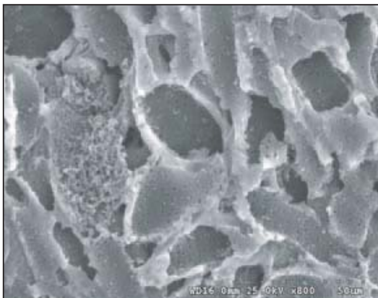
Figure 6. Scanning electron microscope image of activated carbon pores.
