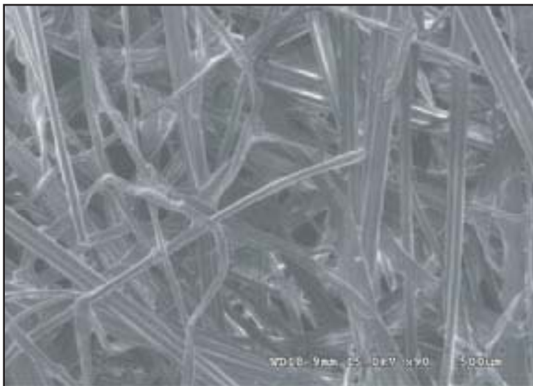
Figure 2. Scanning electron microscope image of a polyester-glass fiber filter.
